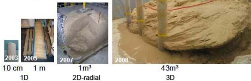
Figure 1 The potential of Biogrout as bio-mediated ground improvement method was assessed using an empirical scale up approach.
